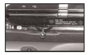
\*Make sure that the adjuster wheel is positive in one of the three detents before firing the rifle.
