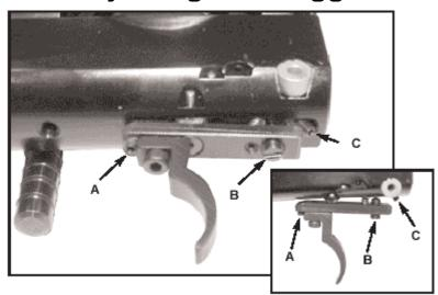
The trigger is factory set for safe usage, however, should you wish to alter the factory settings the mechanism is fully adjustable. To adjust the trigger, firstly remove the action from the stock.
